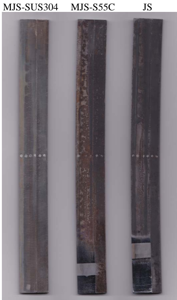
Figure 12: Appearance of quenched JS and MJS specimens.
